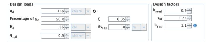
Should it be necessary to define an eccentric load application of  $q_d$ , the input of  $e_{qd}$  can be displayed by pressing the button  $\bullet$ .
