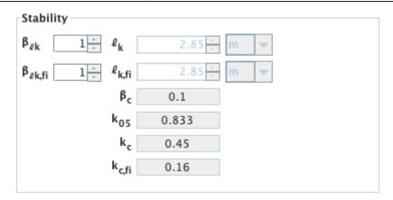
The straightness factor  $\beta_c$  and the conversion factor to the 5% quantile  $k_{05}$  can be changed in the settings.
