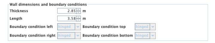
The bearing of the wall at the top and bottom edges is hinged and the lateral edges are free. These boundary conditions cannot be changed at present.
