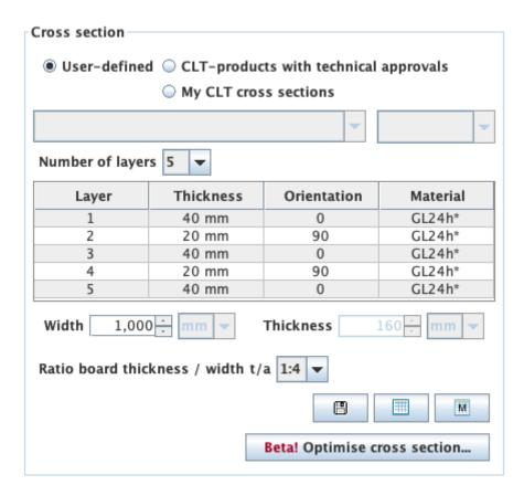
The width of the CLT plate strips can be also defined in this field. The default value is set to 1 m. The thickness of the CLT plate is calculated automatically based on the thickness of the single layers.
