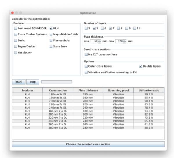
With the help of this tool, the possible layups can be determined for the given system and load situation. The optimization can be restricted with regard to producers, number of layers or by means of limits for the panel thickness. Furthermore, outer cross layers or double layers can be included or excluded. With the option "Vibration verification according to EN" the base document is included in
