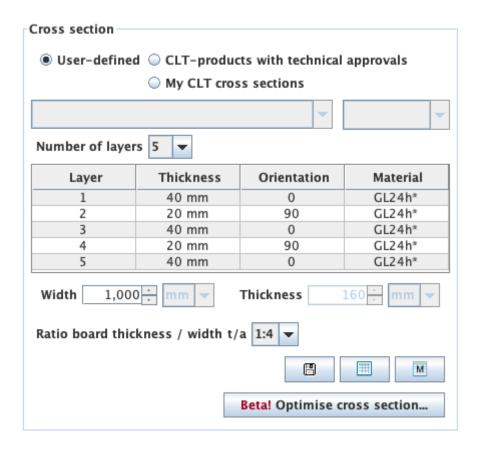
The width of the CLT plate strips can be also defined in this field. The default value is set to 1 m. The
