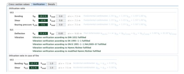
The tab "Utilisation" shows the distribution of the governing utilisation ratios along the beam. Areas in which the results may differ from the exact solution are marked here.
