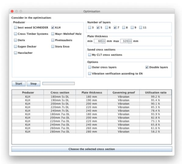
With the help of this tool, the possible layups can be determined for the given system and load situation. The optimization can be restricted with regard to producers, number of layers or by means of limits for the panel thickness. Furthermore, outer cross layers or double layers can be included or excluded. With the option "Vibration verification according to EN" the base document is included in the vibration check or not.
