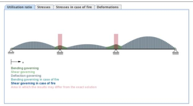
The tab "Stresses" shows the governing stresses resulting from the ULS verification. If a structural fire design was carried out, the governing stresses in case of fire are shown in the tab "Stresses in case of fire"
