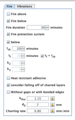
For a user-defined cross section, options are given for specifying heat resistant adhesives, presence of grooves, and whether the layers are edge-glued. For CLT products both values are set automatically and they cannot be changed.
